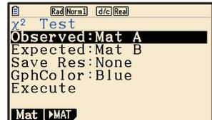
Press **F2** (▶MAT), make sure **Mat A** is highlighted, then press **F3** (DIM) **2** **EXE** **2** **EXE** **EXE**. This indicates that the contingency table has 2 rows and 2 columns.
