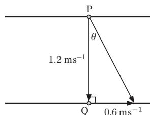
$$\begin{aligned} (\text{actual speed})^2 &= (\text{swimming speed})^2 + (\text{current})^2 \\ &= 1.2^2 + 0.6^2 \\ &= 1.8 \end{aligned}$$
